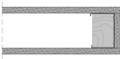
Timber insert into fermacell™ stud opening
