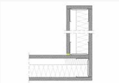
Steel stud corner junction - Filler & glue
