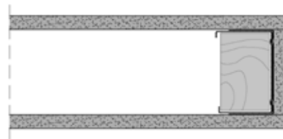
Timber insert into fermacell™ stud opening, with full wrap of track up the door jamb stud.
